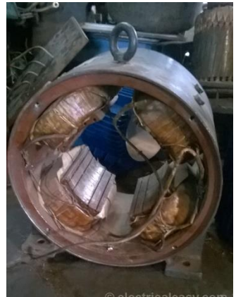
Figure 1.2 Stator of a DC machine
